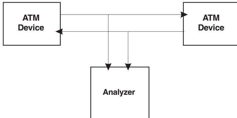
Figure 10-3. Monitoring Between ATM Devices.
