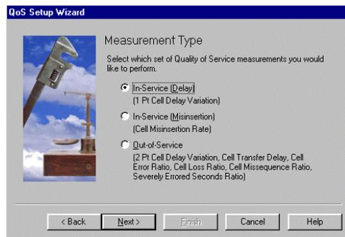
Figure 6-2. The Measurement Type Page of the QoS Setup Wizard
