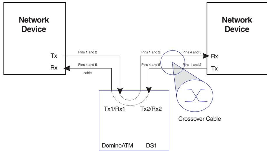
Figure 11-6. Monitoring with the DS1 ATM Interface Module Using RJ-48C Connectors and a Crossover Network
