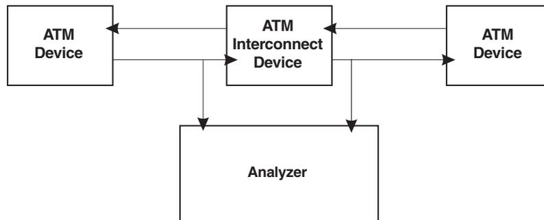
Figure 7-4. Monitoring Across ATM Interconnect Devices.
