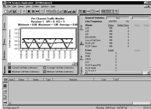
Figure 5-2. The General Statistics View and Per Channel Statistics View (Using E1)
