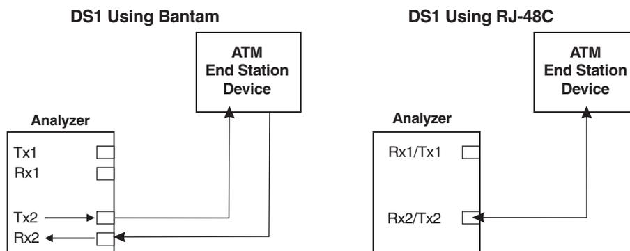
Figure 11-2. Connecting for Emulation for an ATM Network Device (loopback not shown)
