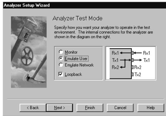
Figure 5-1. The Analyzer Test Mode Page of the Analyzer Setup Wizard
