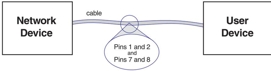
Figure 8-7. Example of a Network Using a 155 UTP Straight-through Cable.
