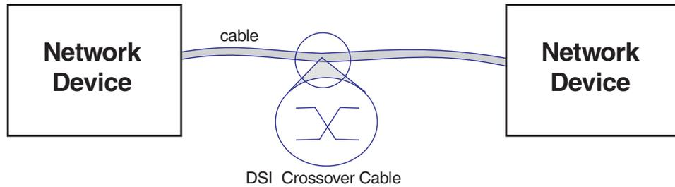
Figure 11-5. Example of a network using a DS1 crossover cable (network to network).
