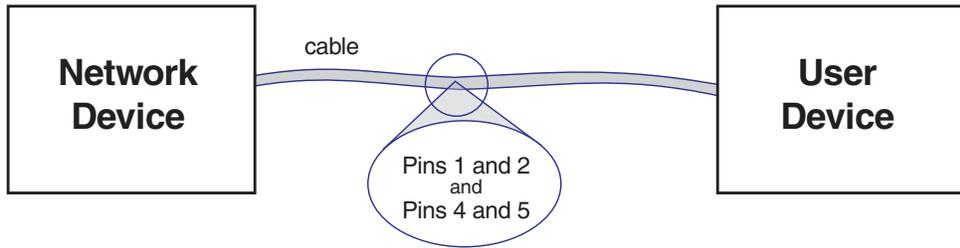
Figure 11-7. Example of a Network Using a DS1 Straight-through Cable (network to user).
