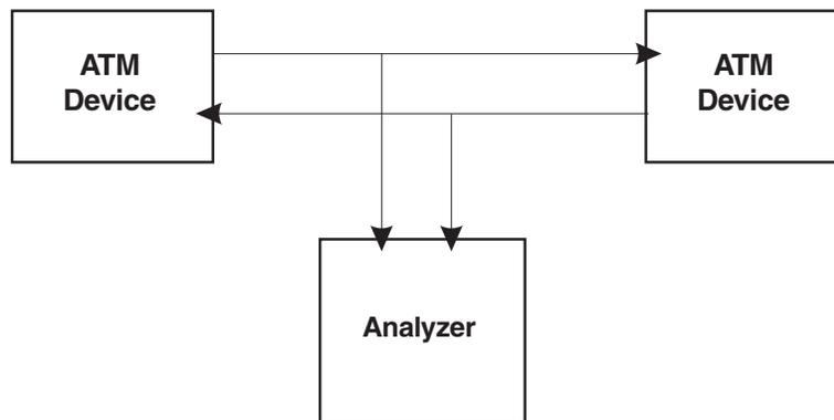
Figure 11-3. Monitoring Between ATM Devices.
