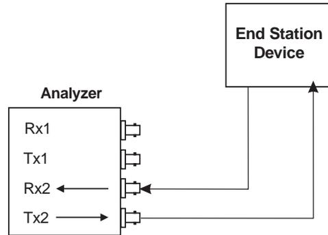
Figure 12-2. Connecting for Emulation for an ATM Network Device (loopback not shown)
