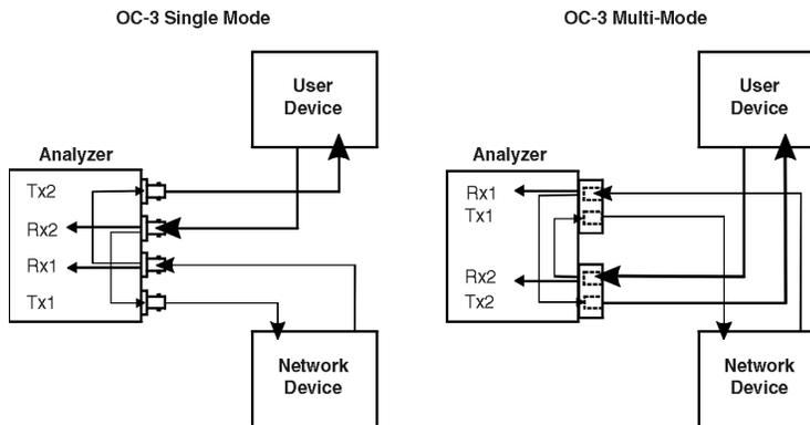
Figure 7-6. Out-of-service Monitoring with the OC-3/STM-1 Interface Modules.
