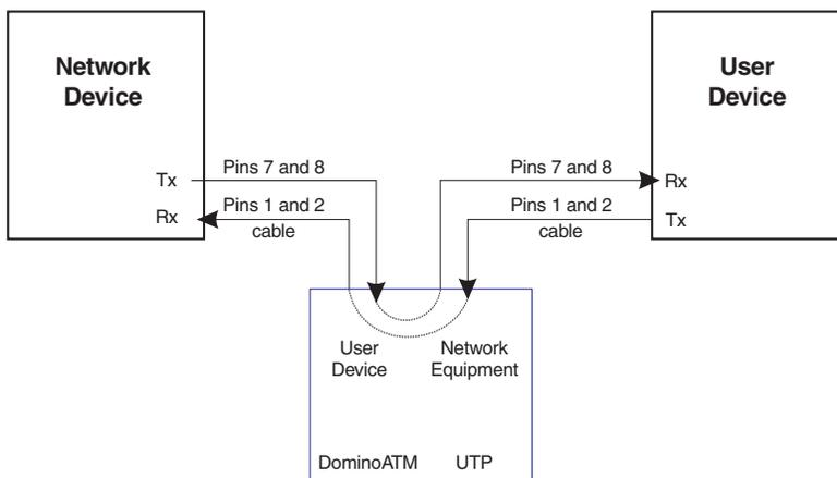
Figure 8-8. Monitoring with the 155 UTP Using RJ-48C and Straight-Through Cables
