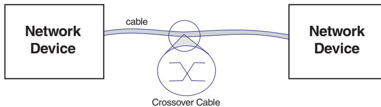
Figure 8-5. Example of a network using a 155 UTP crossover cable.
