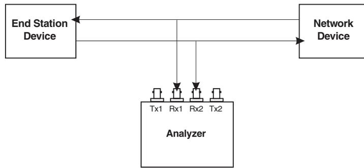
Figure 7-5. In-service monitoring with an OC-3/STM-1 Interface Module (Multi-mode)
