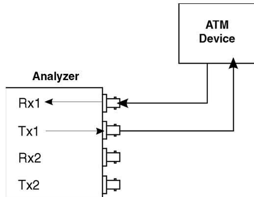
Figure 12-1. Connecting for Emulation for an ATM End Station
