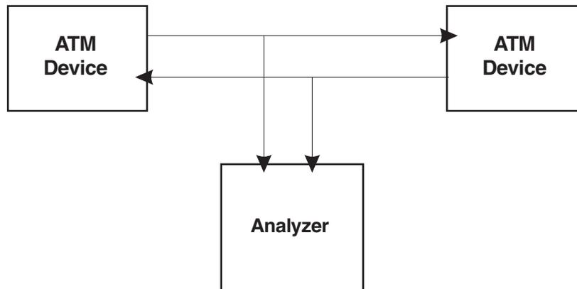
Figure 13-1. Monitoring Between ATM Devices.
