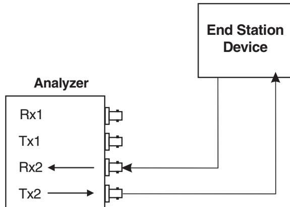
Figure 10-2. Connecting for Emulation for an ATM Network Device (loopback not shown)
