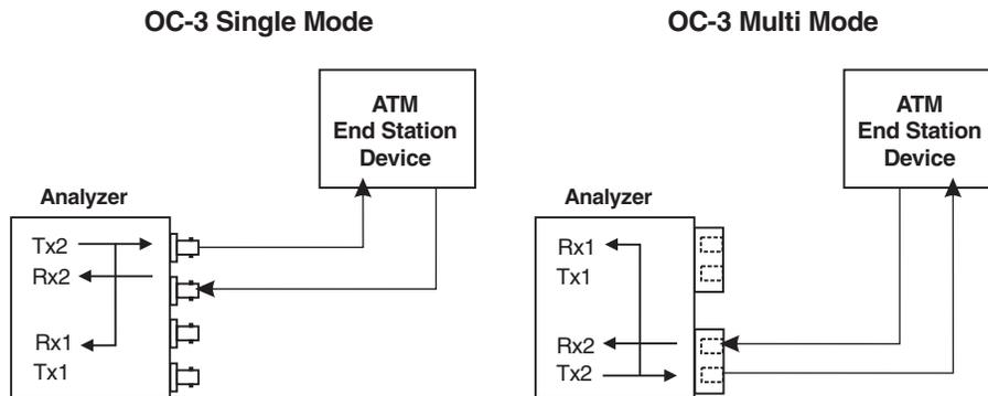
Figure 7-2. Connecting for Emulation for an ATM Network Device (Loopback Shown)
