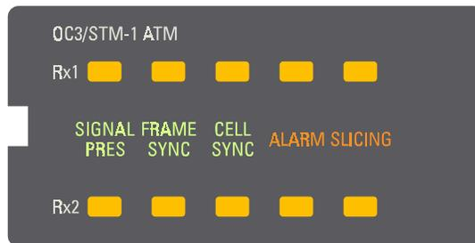
Figure 8-9. The OC-3 LED Overlay Is Used for UTP.
