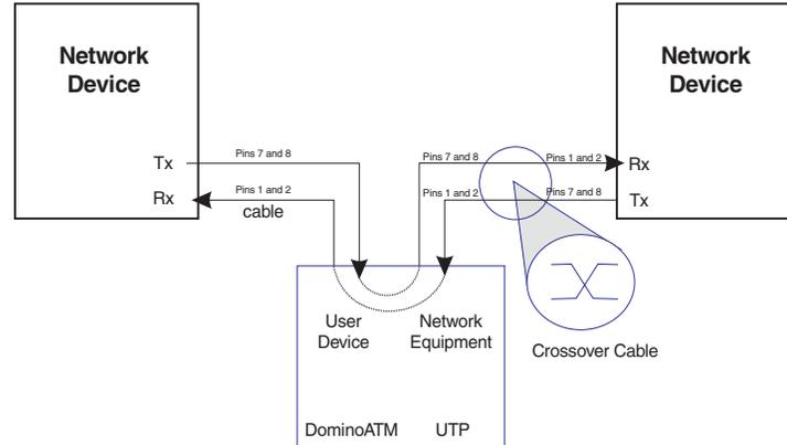
Figure 8-6. Monitoring with the 155 UTP ATM Interface Module Using RJ-48C Connectors and a Crossover Network
