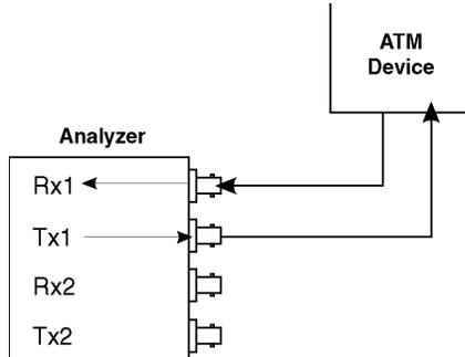
Figure 10-1. Connecting for Emulation for an ATM End Station
