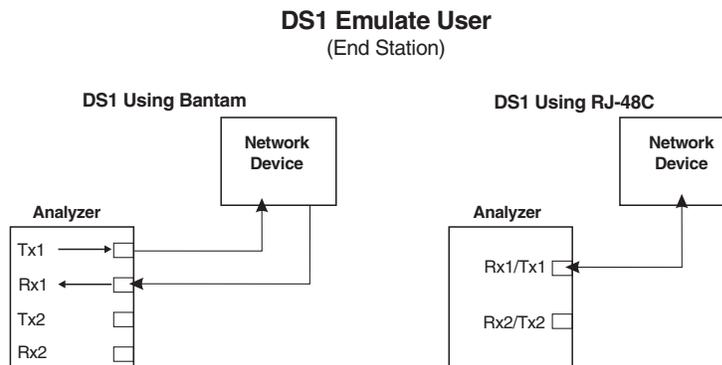
Figure 11-1. Connecting for Emulation for an ATM End Station
