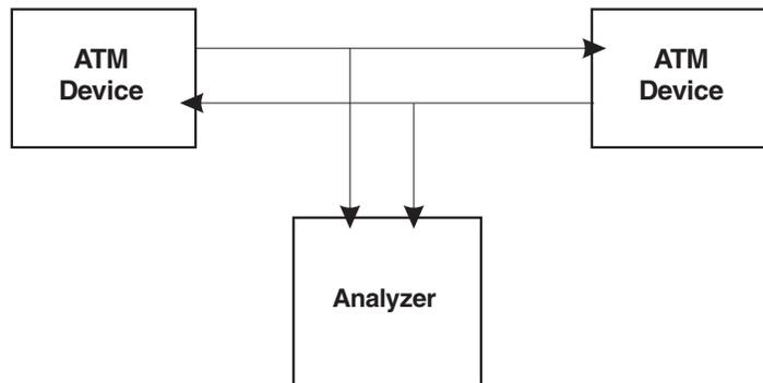
Figure 8-3. Monitoring Between ATM Devices.
