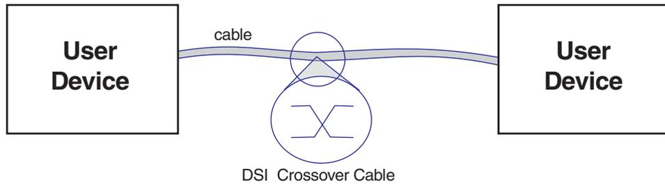
Figure 11-9. Example of a network using a DS1 crossover cable (user to user).
