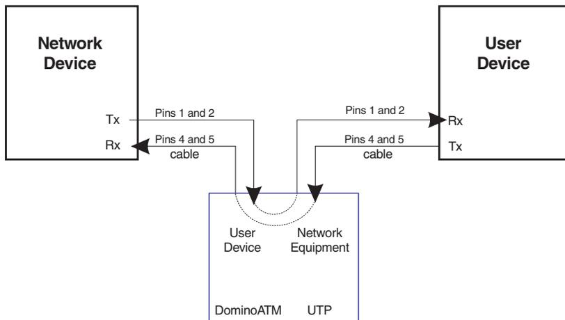
Figure 11-8. Monitoring with the DS1 ATM Interface Module Using RJ-48C and Straight-Through Cables
