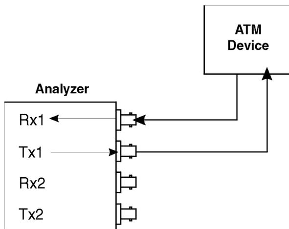
Figure 9-1. Connecting for Emulation for an ATM End Station
