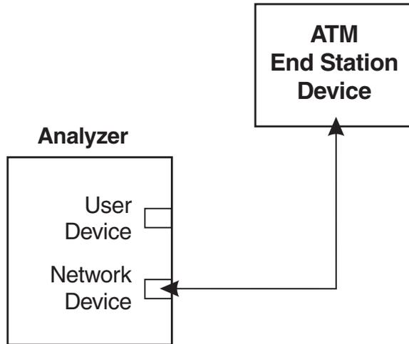
Figure 8-2. Connecting for Emulation for an ATM Network Device (straight-through cable)
