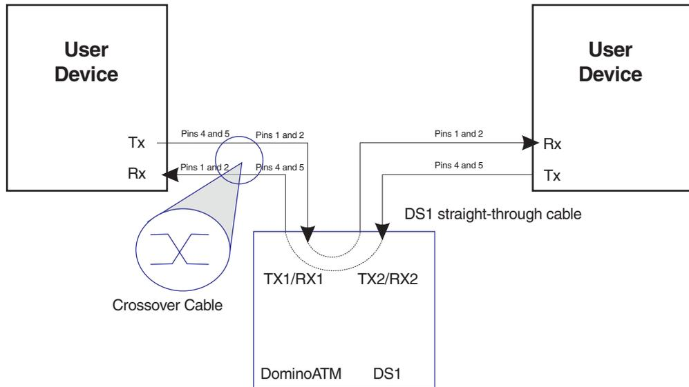
Figure 11-10. Monitoring with the DS1 ATM Interface Module Using RJ-48C Connectors and a Crossover Network
