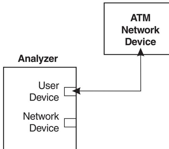
Figure 8-1. Connecting for Emulation for an ATM End Station (straight-through cable)
