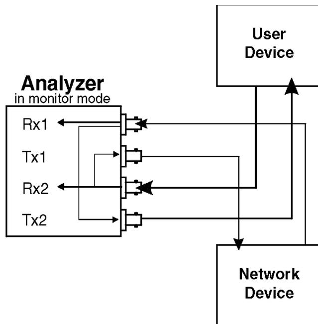
Figure 10-5. E3 ATM Interface Module Monitoring Connections
