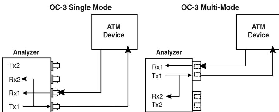
Figure 7-1. Connecting for Emulation for an ATM End Station (Loopback Shown)
