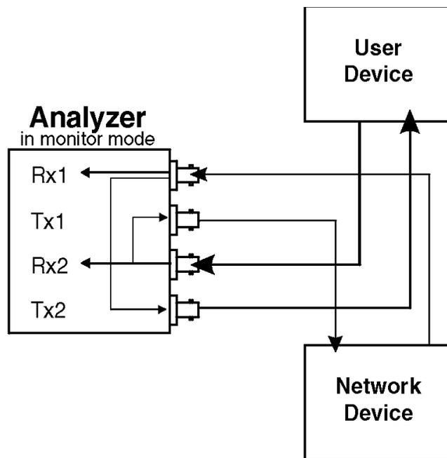
Figure 9-4. E1 ATM Interface Module Monitoring Connections
