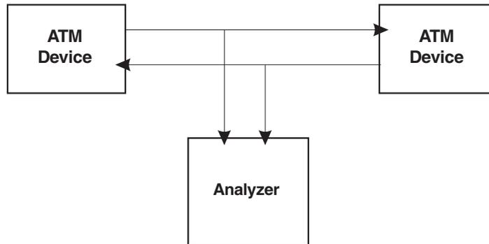
Figure 7-3. Monitoring Between ATM Devices.
